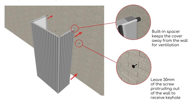
Drive the wall plug and screws in, leaving 30mm protruding out of the wall. Let the screw follow the path of the red dotted line shown below.
